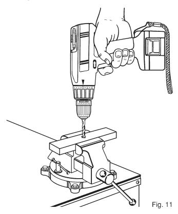
When drilling hard smooth surfaces use a center punch to mark desired hole location. This will prevent the drill bit from slipping off center as the hole is started. However, the low speed feature allows starting holes without center punching if desired. To accomplish this, simply operate your drill at a low speed until the hole is started.
